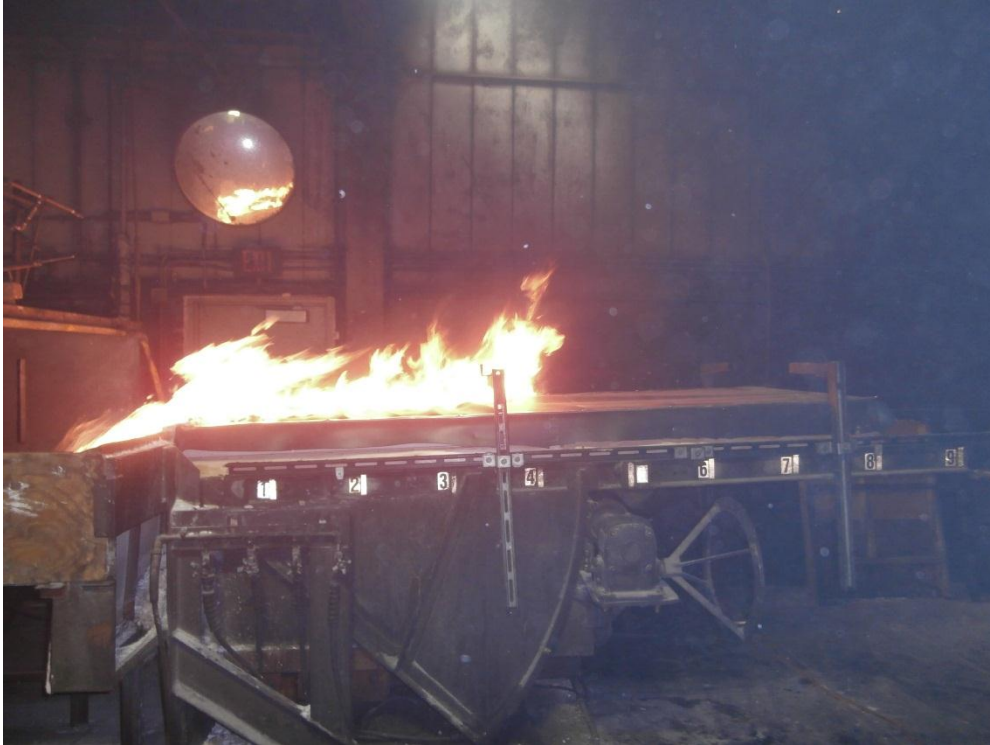
Figure 3 – Figure Illustrating Flame Spread of System 3 (No PV Module)
