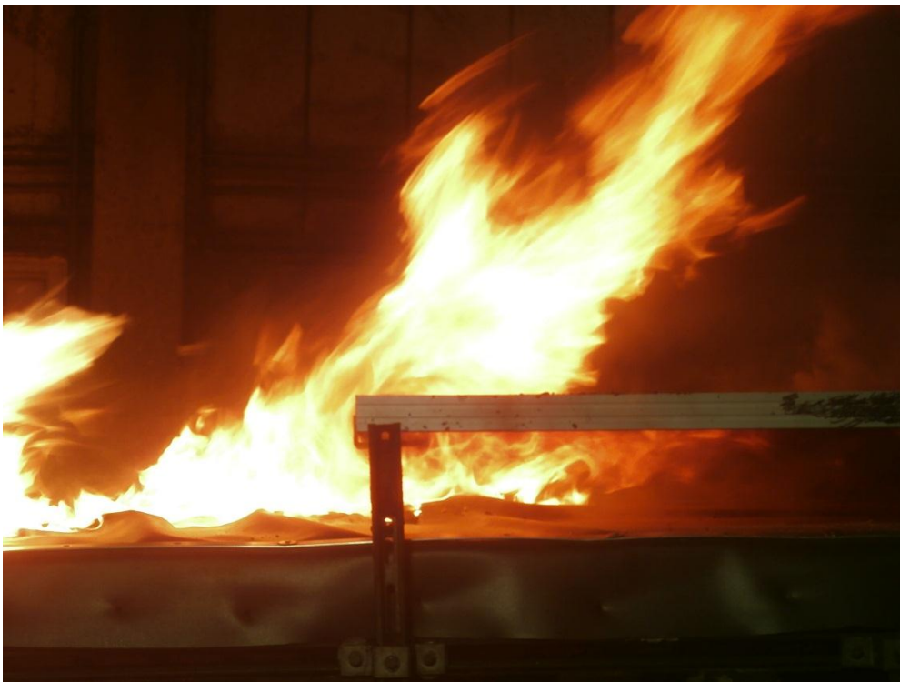
Figure 4 – Figure Illustrating Ignition of the Module and Roof of System 4
