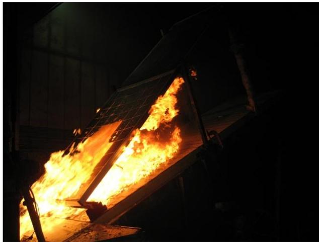
**Figure 19 – System 9 Spread of Flame Test with PV Module Mounted 22° to Steep Sloped Roof (Positive)**
