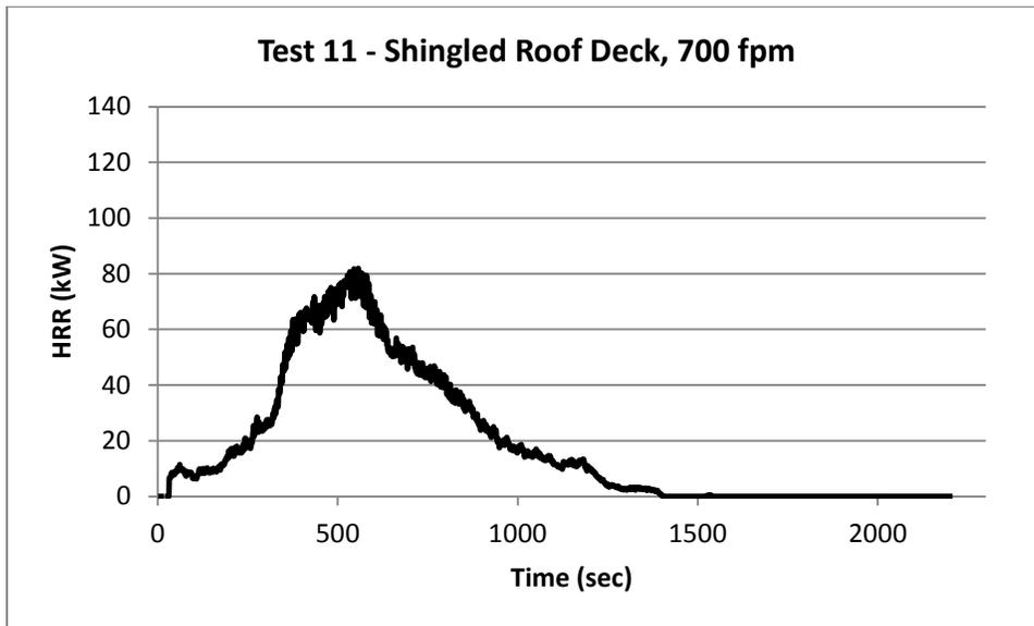
Figure 55 - Graph of Heat Release Rate (HRR) in kilowatts
