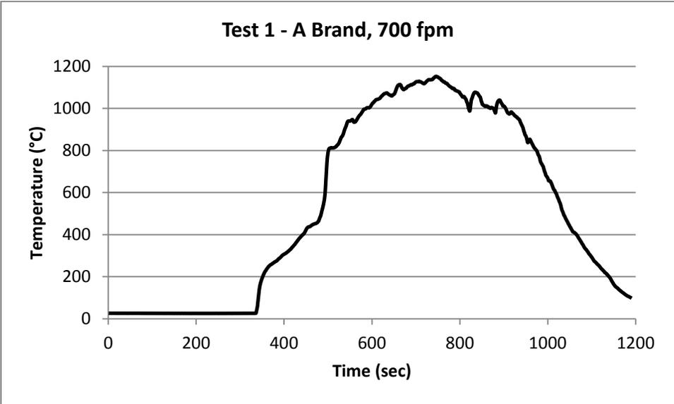
**Figure 32 - Graph of Deck Surface Temperature (°C)**
