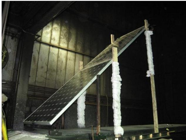
**Figure 10 – System 5 Spread of Flame Test PV with PV Module Mounted 45° to Low Sloped Roof (Positive) Set Up**
