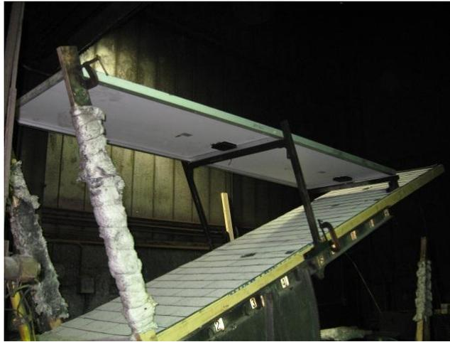
**Figure 20 – System 10 Spread of Flame Test with PV Module Mounted 22° to Steep Sloped Roof (Negative) Set Up**
