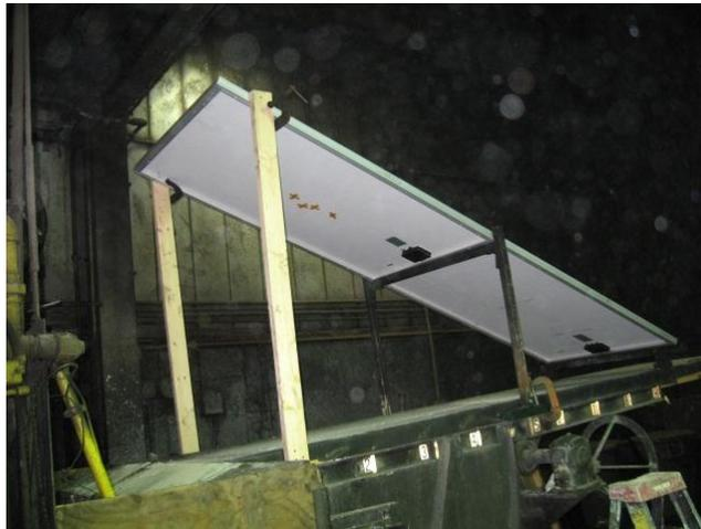
**Figure 12 – System 6 Spread of Flame Test PV with PV Module Mounted 45° to Low Sloped Roof (Negative) Set Up**
