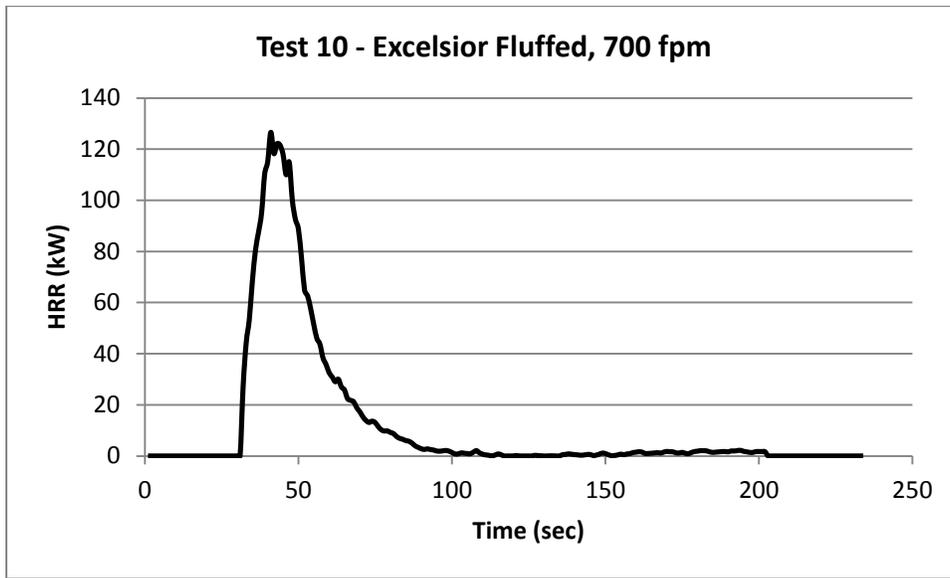
Figure 53 - Graph of Heat Release Rate (HRR) in kilowatts
