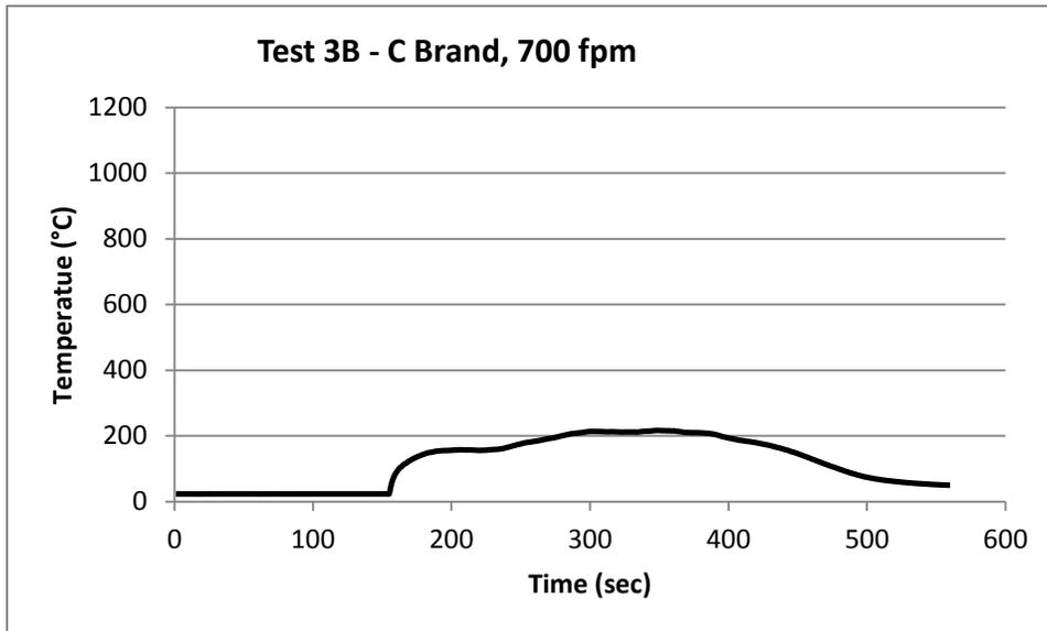
Figure 38 - Graph of Deck Surface Temperature (°C)
