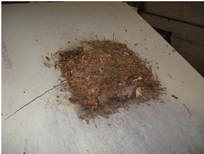
**Figure 27 - Leave Debris Over Noncombustible Deck Set Up**
