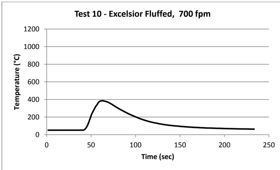
Figure 54 - Graph of Deck Surface Temperature (°C)
