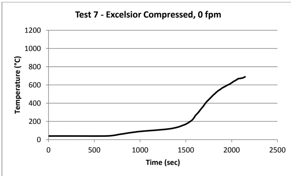
Figure 48 - Graph of Deck Surface Temperature (°C)
