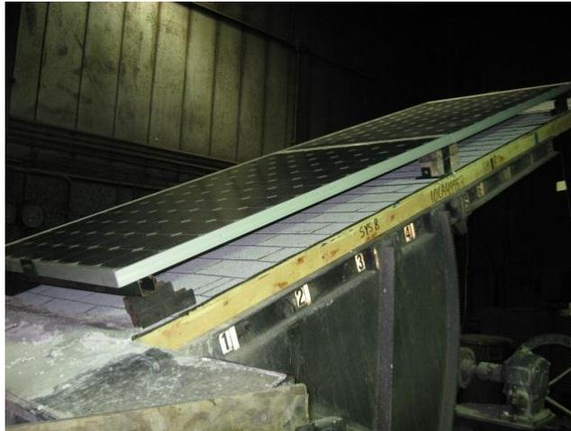
**Figure 16 – System 8 Spread of Flame Test PV Module Mounted Parallel to Steep Sloped Roof, 5” Gap Set Up**
