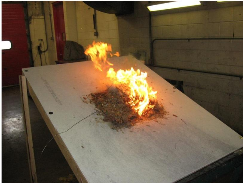
**Figure 28 - Leave Debris Over Noncombustible Deck**
