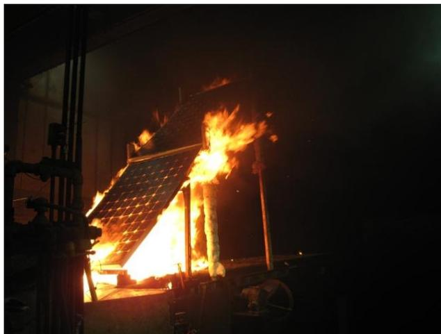
**Figure 11 – System 5 Spread of Flame Test PV with PV Module Mounted 45° to Low Sloped Roof (Positive)**
