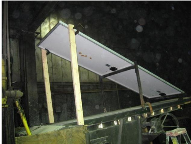
**Figure 14 – System 7 Spread of Flame Test PV with PV Module Mounted 22° to Low Sloped Roof with 2” Polyisocyanurate Foam (Negative) Set Up**
