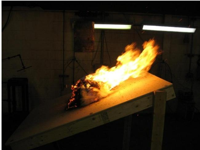
**Figure 26 - Class Wood Excelsior Over Noncombustible Deck**
