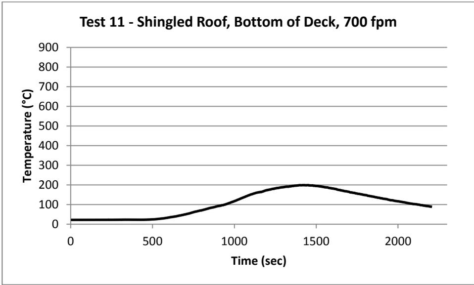
**Figure 59 - Graph of Underside of Deck Surface Temperature (°C)**
