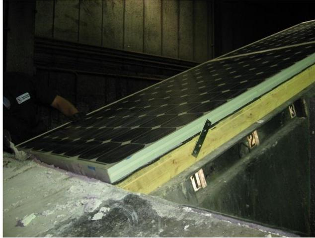
**Figure 2 – System 1 Spread of Flame Experiment with PV Modules Mounted Directly to Shingled Deck, Ignition Source Directed at Roof Surface Set Up**
