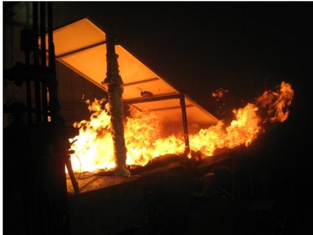
**Figure 15 – System 7 Spread of Flame Test PV with PV Module Mounted 22° to Low Sloped Roof with 2” Polyisocyanurate Foam (Negative)**
