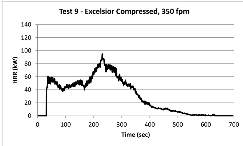
Figure 51 - Graph of Heat Release Rate (HRR) in kilowatts
