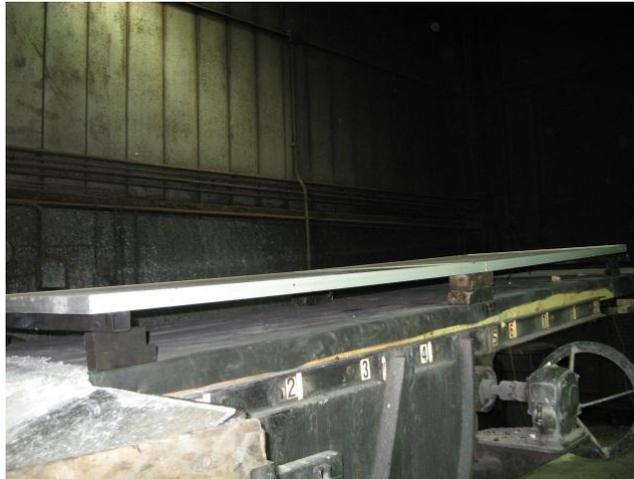
**Figure 6 – System 3 Spread of Flame Test PV with Module Mounted Parallel to Low Sloped Roof, 5” Gap Set Up**
