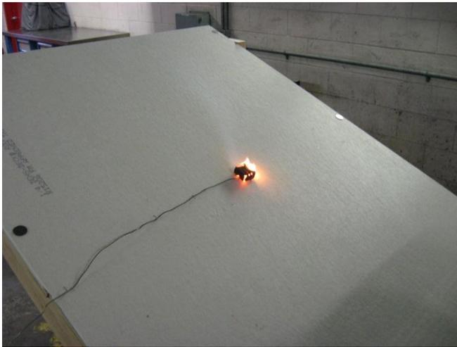
**Figure 24 - Class C Brand Over Noncombustible Deck**
