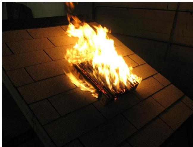
**Figure 29 - Class A Brand Over Shingled Combustible Deck**
