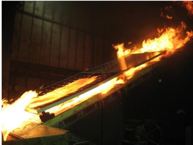
**Figure 17 – System 8 Spread of Flame Test PV Module Mounted Parallel to Steep Sloped Roof, 5” Gap**
