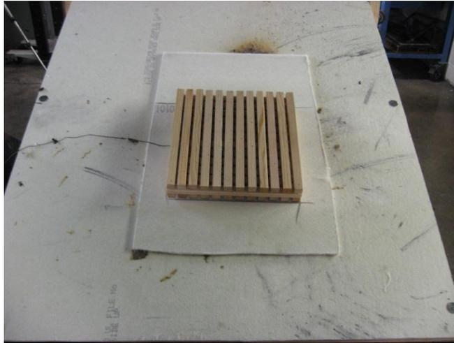
**Figure 22 - Class A Brand Over Noncombustible Deck Set Up**
