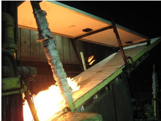
**Figure 21 – System 10 Spread of Flame Test with PV Module Mounted 22° to Steep Sloped Roof (Negative)**
