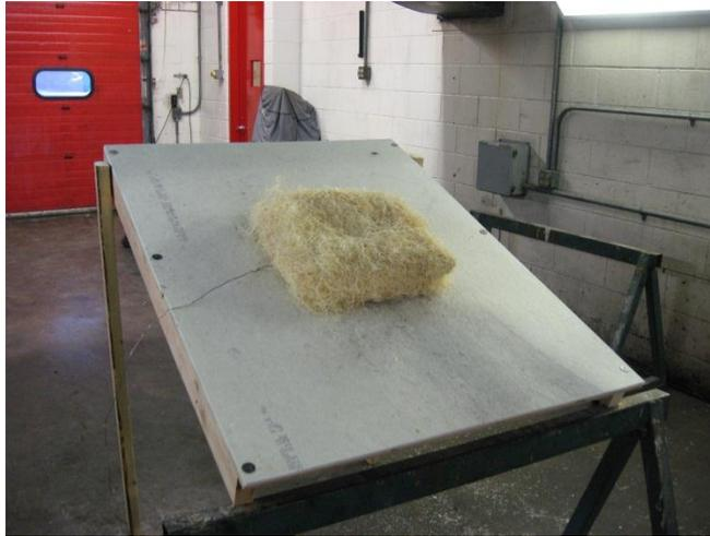
**Figure 25 - Class Wood Excelsior Over Noncombustible Deck Set Up**
