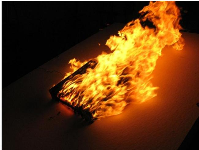
**Figure 23 - Class A Brand Over Noncombustible Deck**
