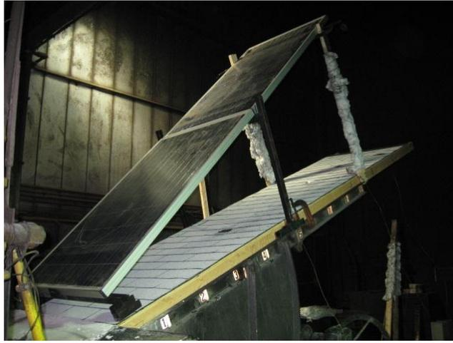
**Figure 18 – System 9 Spread of Flame Test with PV Module Mounted 22° to Steep Sloped Roof (Positive) Set Up**
