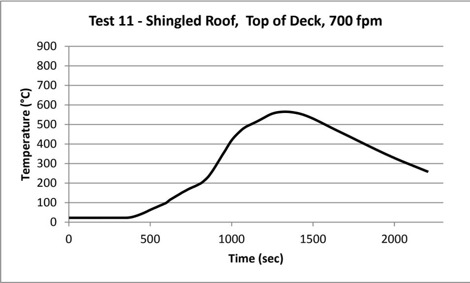
**Figure 58 - Graph of Deck Surface Temperature (°C)**
