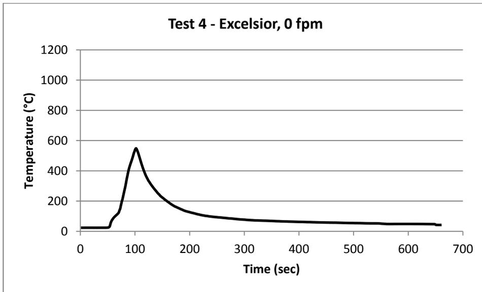
Figure 42 - Graph of Deck Surface Temperature (°C)
