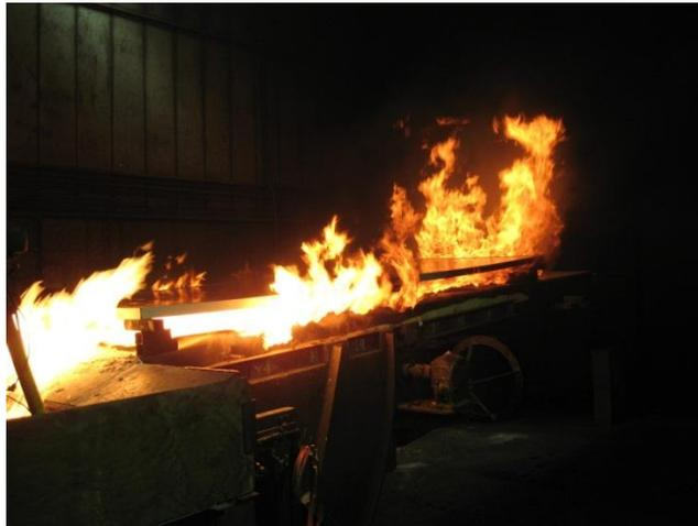
**Figure 7 – System 3 Spread of Flame Test PV with Module Mounted Parallel to Low Sloped Roof, 5” Gap**
