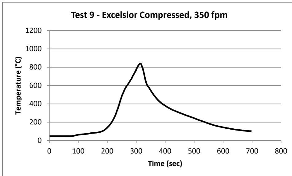
Figure 52 - Graph of Deck Surface Temperature (°C)
