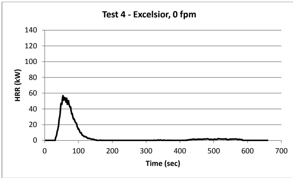
Figure 41 - Graph of Heat Release Rate (HRR) in kilowatts
