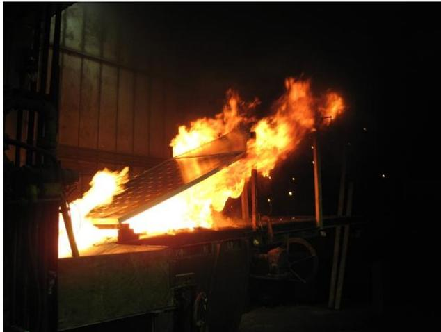
**Figure 9 – System 4 Spread of Flame Test PV with PV Module Mounted 22° to Low Sloped Roof (Positive)**
