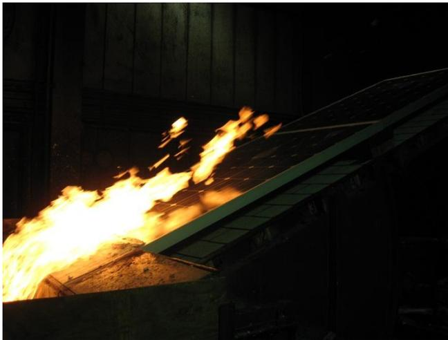
**Figure 5 – System 2 Spread of Flame Experiment with PV Modules Mounted Directly to Shingled Deck, Ignition Source Directed at PV Superstrate Surface**
