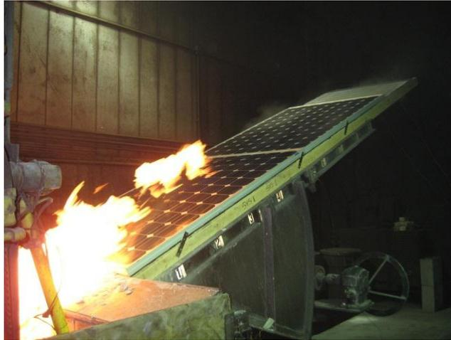
**Figure 3 –System 1 Spread of Flame Experiment with PV Modules Mounted Directly to Shingled Deck, Ignition Source Directed at Roof Surface**
