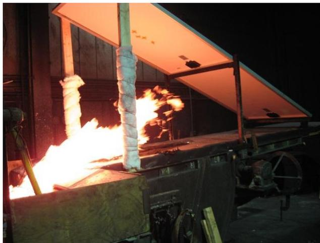
**Figure 13 – System 6 Spread of Flame Test PV with PV Module Mounted 45° to Low Sloped Roof (Negative)**
