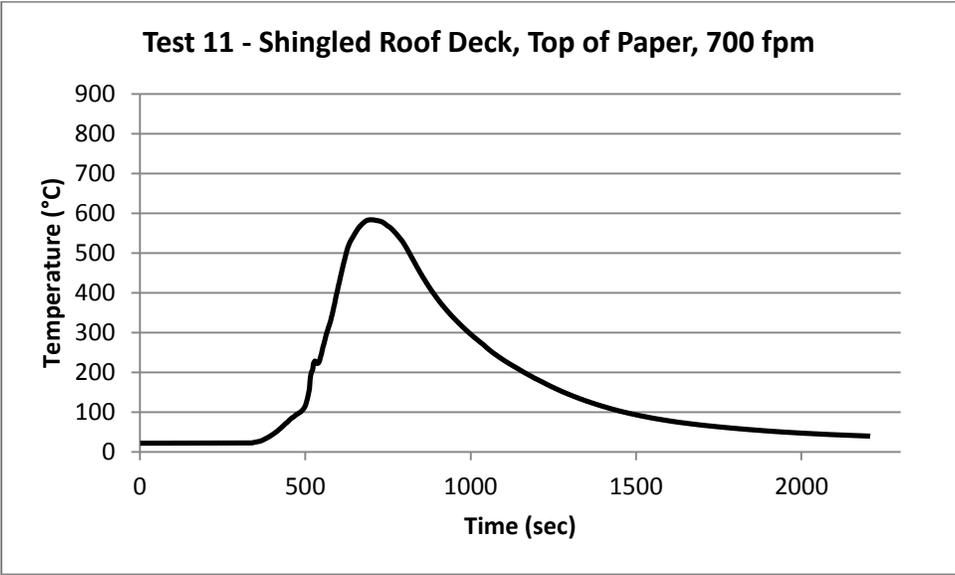
**Figure 57 - Graph of Tar Paper Surface Temperature (°C)**
