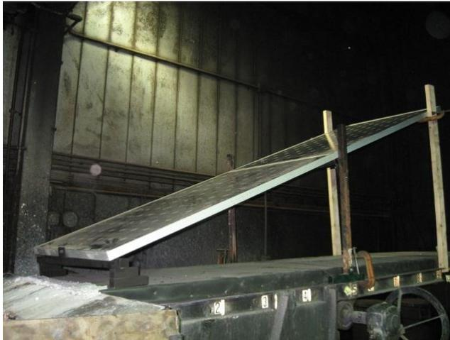
**Figure 8 – System 4 Spread of Flame Test PV with PV Module Mounted 22° to Low Sloped Roof (Positive) Set Up**
