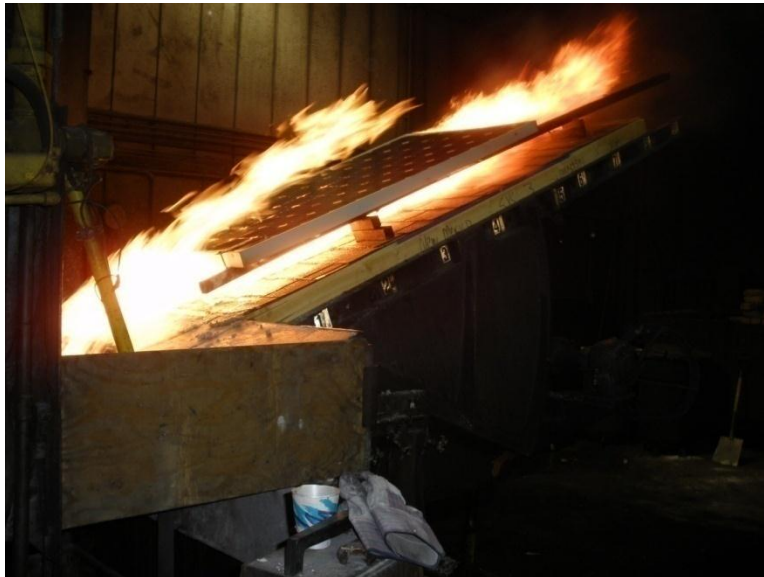
Figure 44 Photograph of Spread of Flame for Class A Laminated (Architectural) Shingle Roof with Class C PV with 0" Leading Edge and 5" Gap
