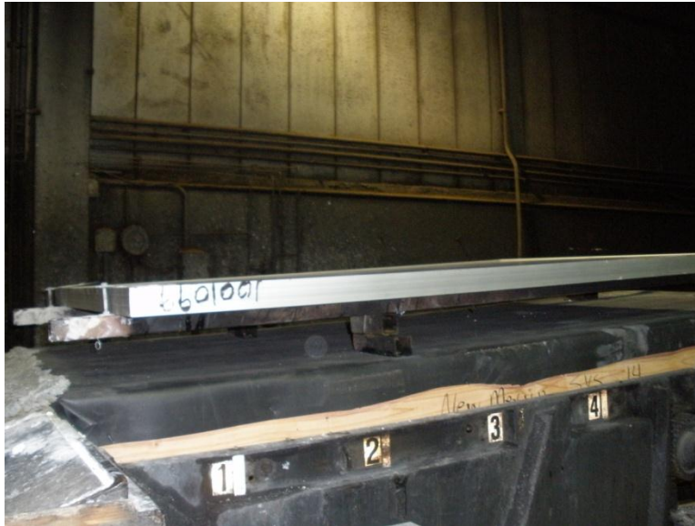
Figure 45 Photograph of Spread of Flame for Class A Built Up Roof (Hot Mopped Asphalt) with Class C PV and 0" Leading Edge and 5" Gap – before start of experiment
