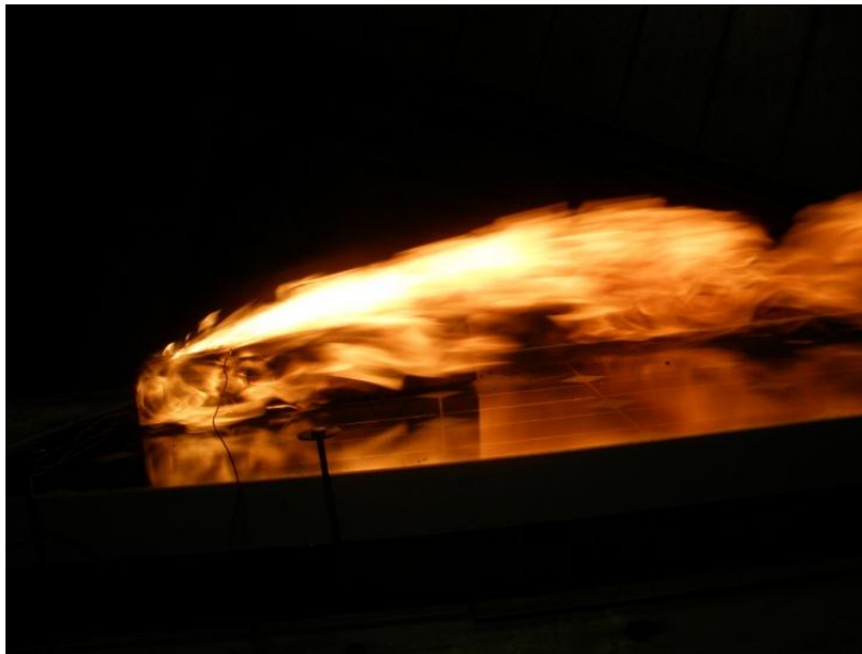
Figure 32 Photograph of Burning Brand on Module for Class A Shingle Roof with Class C PV and 0” Gap
