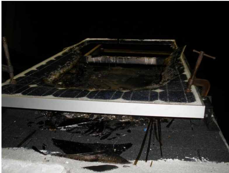
Figure 38 Photograph of Burning Brand between Module and Roof for Class A Shingle Roof with Class C PV and 5" Gap
