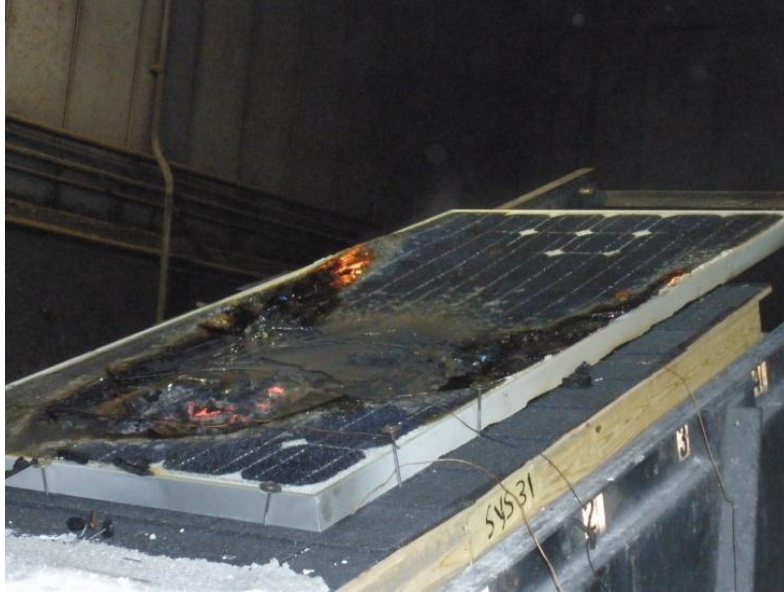
Figure 33 Photograph of Burning Brand on Module for Class A Shingle Roof with Class C PV and 0” Gap
