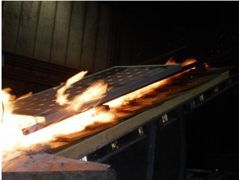
Figure 40 Photograph of Spread of Flame Test for Class C Wood Shake Roof with Class C PV and 0” Leading Edge and 5” Gap
