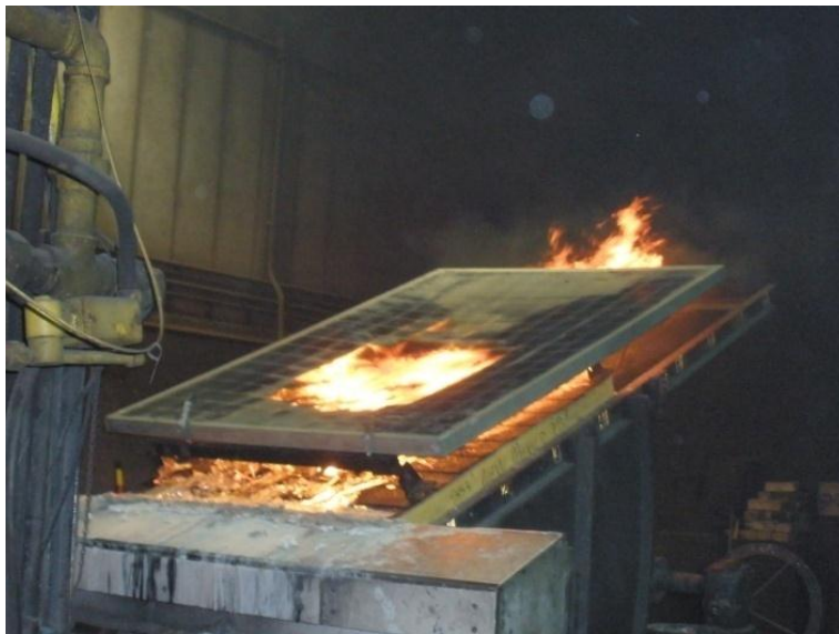
Figure 54 Burning Brand Test for Class A Shingle (3 tab) Roof with Class A PV where Class A brand was located on the surface of the roof under the module
