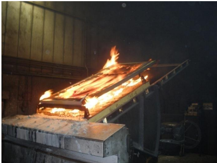
Figure 48 Burning Brand Test for Class A Shingle (3 tab) Roof with Class C PV where Class A brand is located on the surface of the roof under the module
