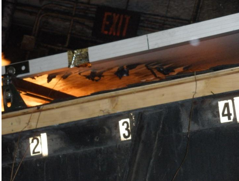
Figure 29 Photograph of Spread of Flame Test for Class A Shingle Roof with Class C PV and Horizontal Mounts and 0" Leading Edge and 5" Gap
