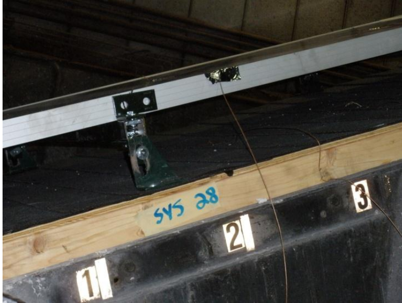
Figure 27 Photograph of Spread of Flame Test for Class A Shingle Roof with Class C PV and Horizontal Mounts and 0" Leading Edge and 5" Gap
