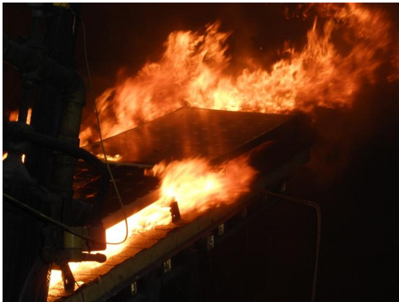
Figure 30 Photograph of Spread of Flame Test for Class A Shingle Roof with Class C PV and Horizontal Mounts and 0" Leading Edge and 5" Gap
