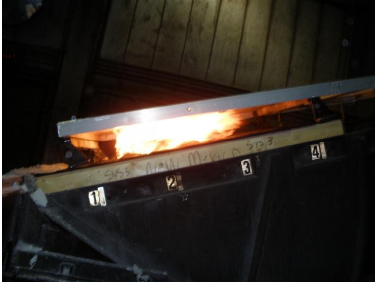
Figure 53 Burning Brand Test for Class A Shingle (3 tab) Roof with Class A PV where Class A brand was located on the surface of the roof under the module
