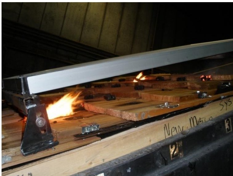
Figure 50 Burning Brand Test for Class C Wood Shake Roof with Class C PV where Class C brand was located on the surface of the roof
