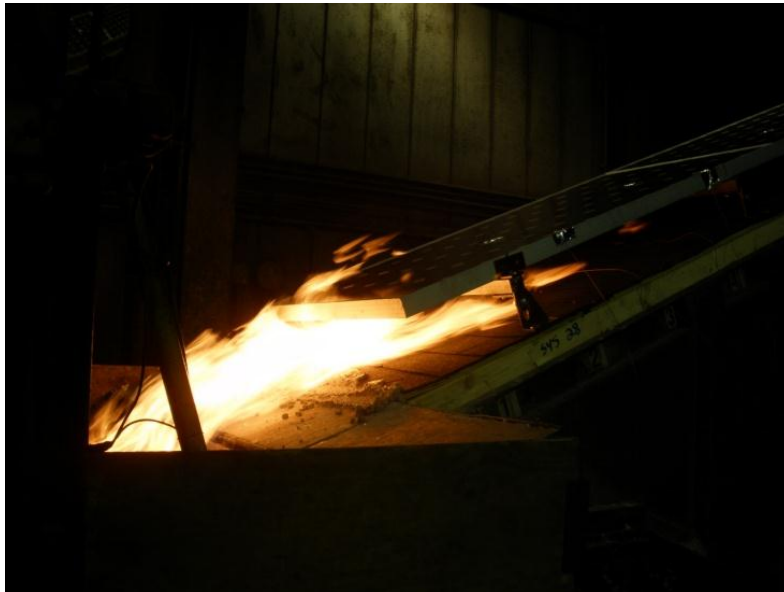
Figure 28 Photograph of Spread of Flame Test for Class A Shingle Roof with Class C PV and Horizontal Mounts and 0" Leading Edge and 5" Gap
