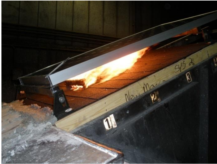
Figure 47 Burning Brand Test for Class A Shingle (3 tab) with Class C PV where Class A brand is located on the surface of the roof under the module
