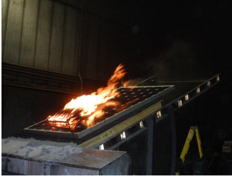
Figure 31 Photograph of Burning Brand on Module for Class A Shingle Roof with Class C PV and 0” Gap
