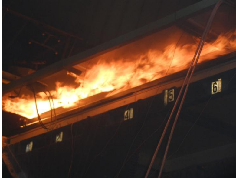
Figure 25 Photograph of Spread of Flame Test for Class A Shingle Roof with Class C PV and Vertical Mounts and 0" Leading Edge and 5" Gap
