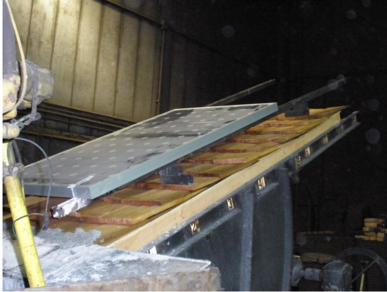
Figure 39 Photograph of Spread of Flame Test for Class C Wood Shake Roof with Class C PV and 0” Leading Edge and 5” Gap – before start of experiment
