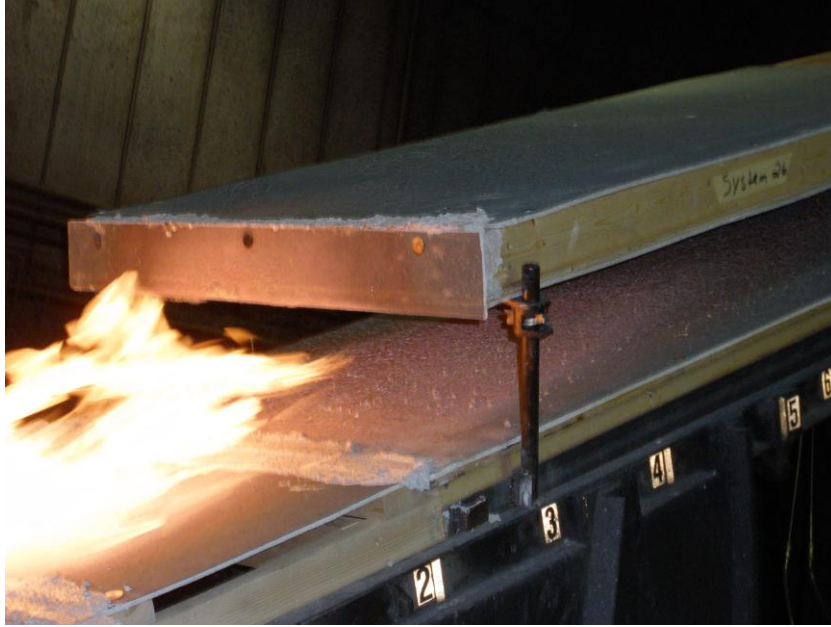
Figure 12 Photograph of Non-combustible Roof and Simulated PV Module Spread of Flame test with 12" Setback and 5" Gap (Assembly 36)
