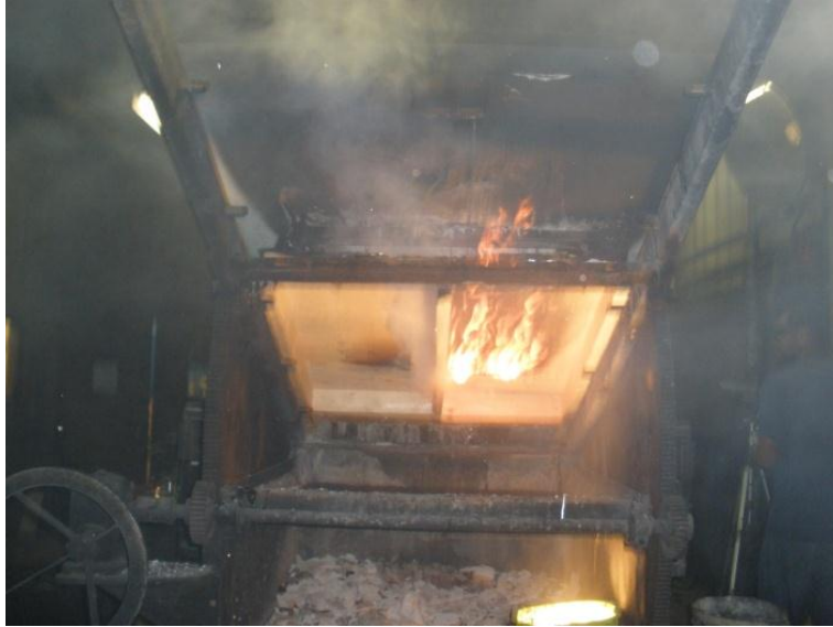
Figure 55 View of Deck Underside: Burning Brand Test for Class A Shingle (3 tab) Roof with Class A PV where Class A brand was located on the surface of the roof under the module
