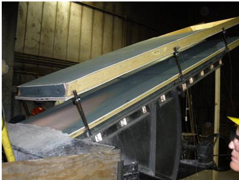
Figure 6 Photograph of Noncombustible PV Module & Roof Deck Test Fixture
