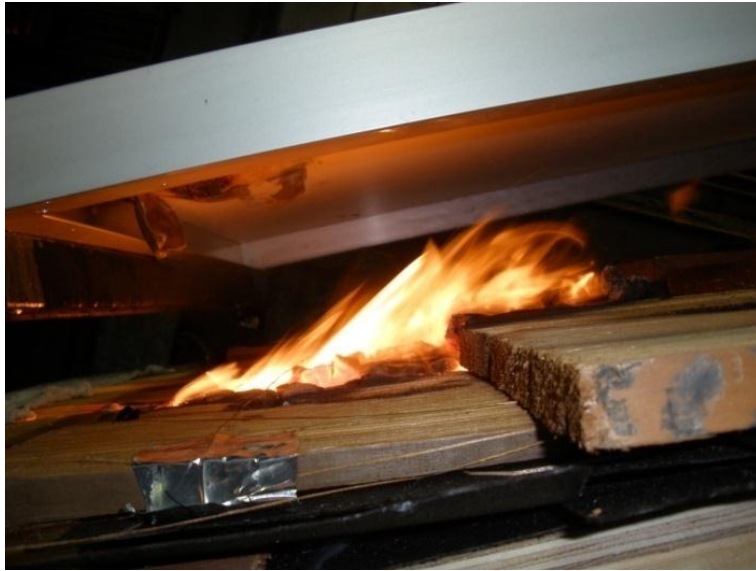
Figure 51 Burning Brand Test for Class C Wood Shake Roof with Class C PV where Class C brand was located on the surface of the roof
