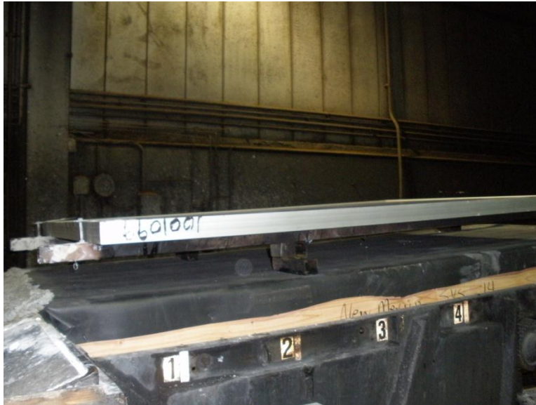
Figure 41 Photograph of Spread of Flame Test for Class A Membrane Roof with Class A PV and 0" Leading Edge and 5" Gap – prior to start of experiment
