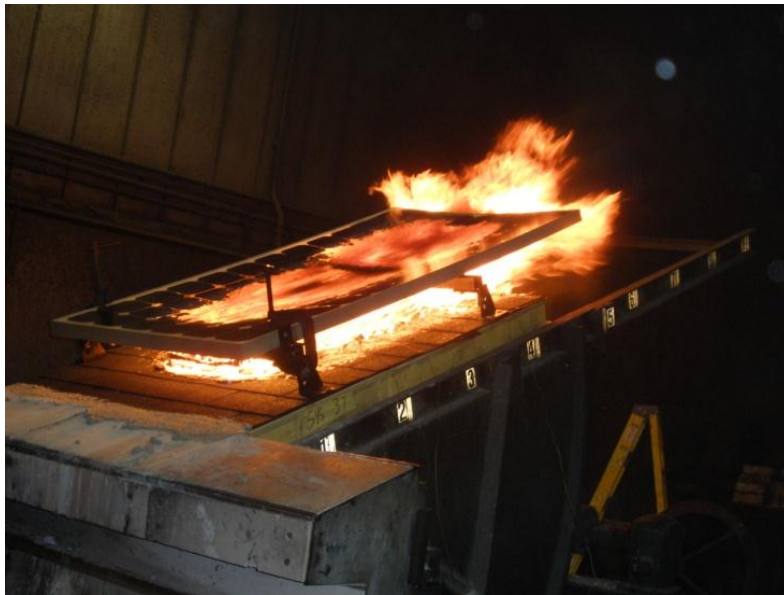
Figure 36 Photograph of Burning Brand Between Module and Roof for Class A Shingle Roof with Class C PV and 5" Gap
