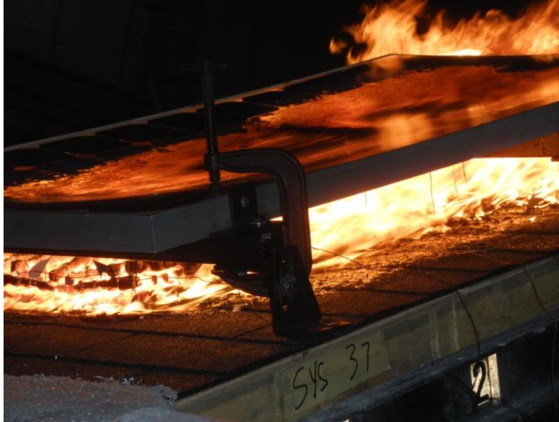
Figure 37 Photograph of Burning Brand between Module and Roof for Class A Shingle Roof with Class C PV and 5" Gap
