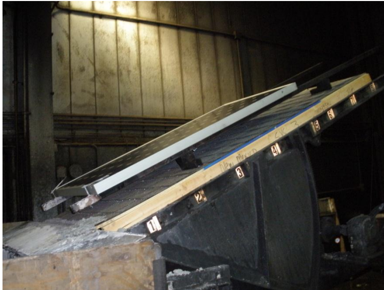
Figure 43 Photograph of Spread of Flame for Class A Laminated (Architectural) Shingle Roof with Class C PV with 0" Leading Edge and 5" Gap – before start of experiment
