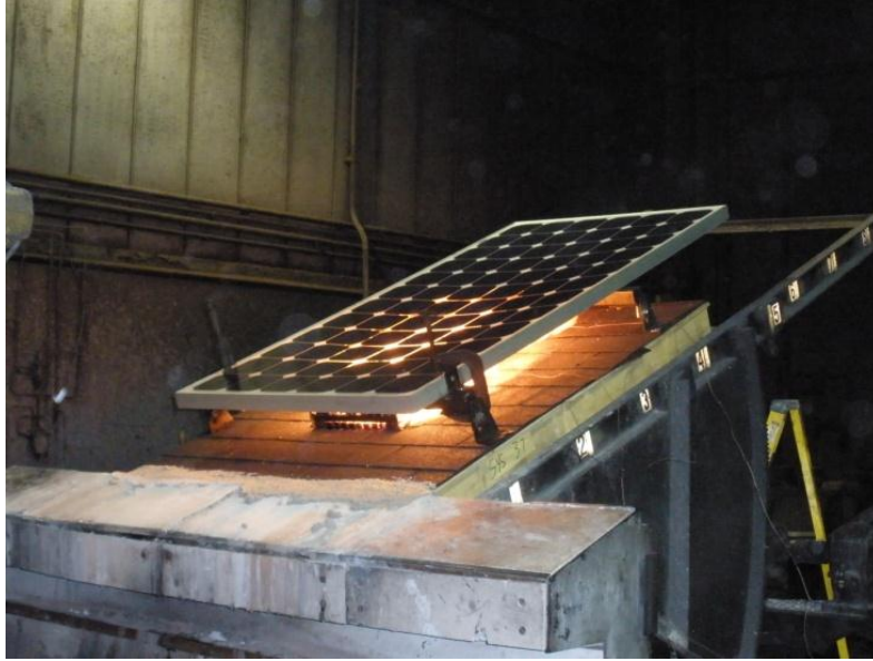
Figure 35 Photograph of Burning Brand Between Module and Roof for Class A Shingle Roof with Class C PV and 5" Gap
