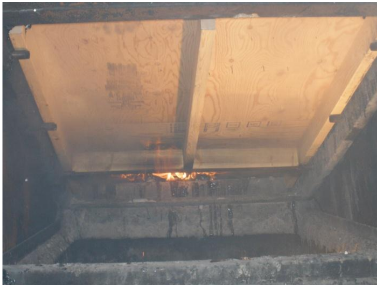
Figure 52 Underside of Roof Deck View: Burning Brand Test for Class C Wood Shake Roof with Class C PV where Class C brand was located on the surface of the roof
