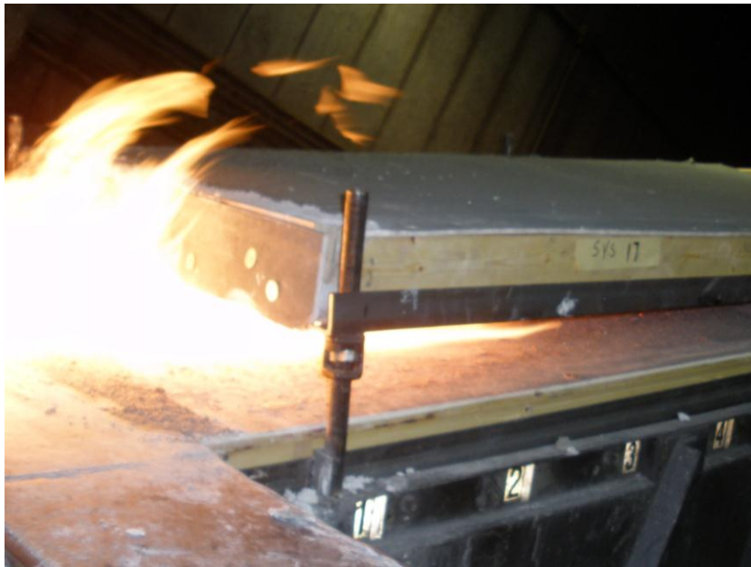
Figure 11 Photograph of non-combustible Roof and Simulated PV Module Spread of Flame test with 0" Setback and 5" Gap (Assembly 12)
