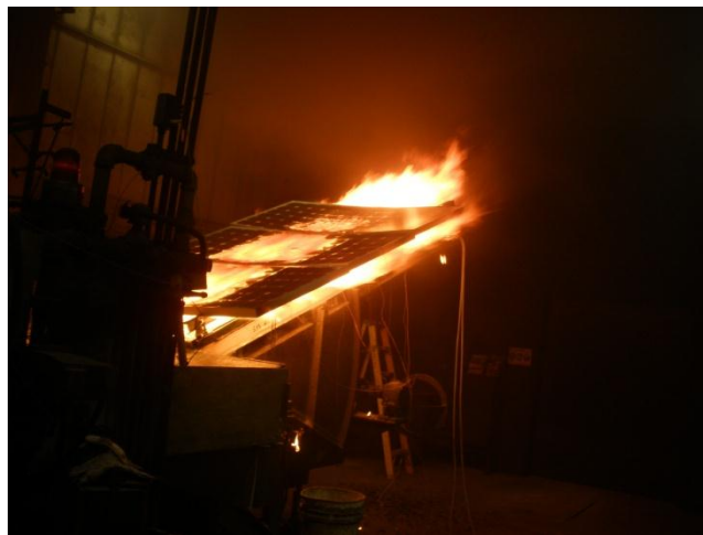
Figure 24 Photograph of Spread of Flame Test for Class A Shingle Roof with Class C PV and Vertical Mounts and 0" Leading Edge and 5" Gap
