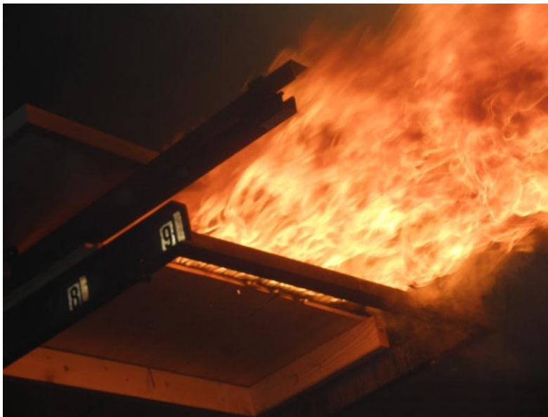
Figure 26 Photograph of Spread of Flame Test of Class A Shingle Roof with Class C PV and Vertical Mounts and 0" Leading Edge and 5" Gap
