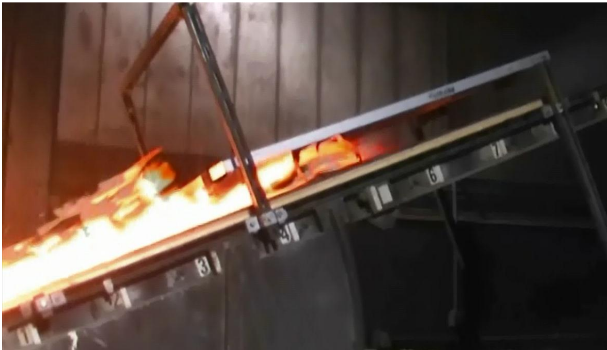
Figure 7 – Figure Illustrating Flame Spread of System 6 – Steep Slope Roof / PV Module Mfg. #3 Shingle, 5" Gap, 0° Inclination and 42" Offset Experiment
