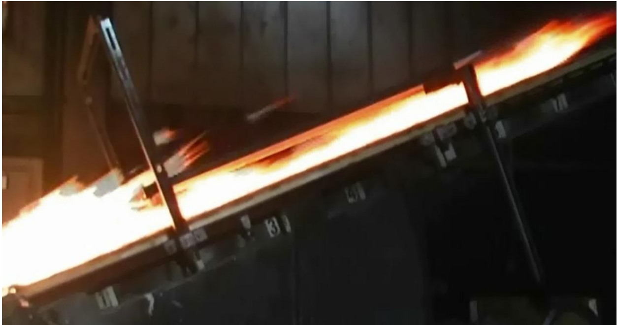
Figure 10 – Figure Illustrating Flame Spread of System 7 – Steep Slope Roof / Noncombustible PV Surrogate Mfg. #2 Shingle, 5" Gap, 0° Inclination and 24" Offset Experiment
