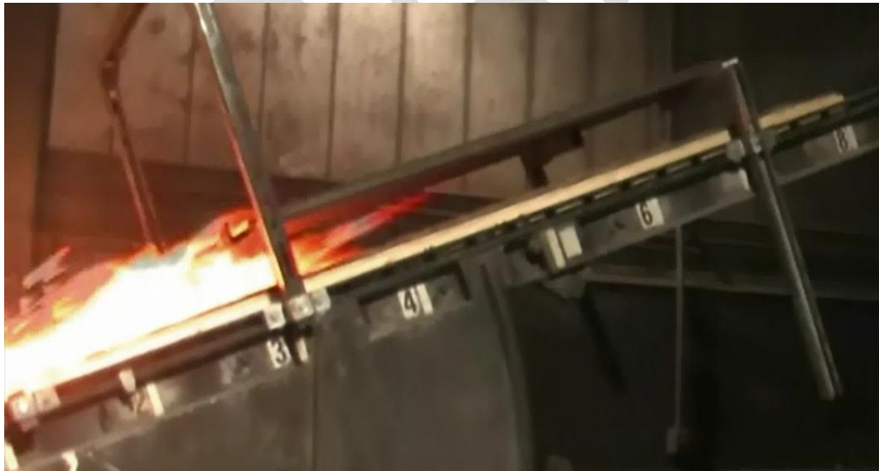
Figure 9 – Figure Illustrating Flame Spread of System 3 – Steep Slope Roof / Noncombustible PV Surrogate Mfg. #1 Shingle, 5" Gap, 0° Inclination and 36" Offset Experiment
