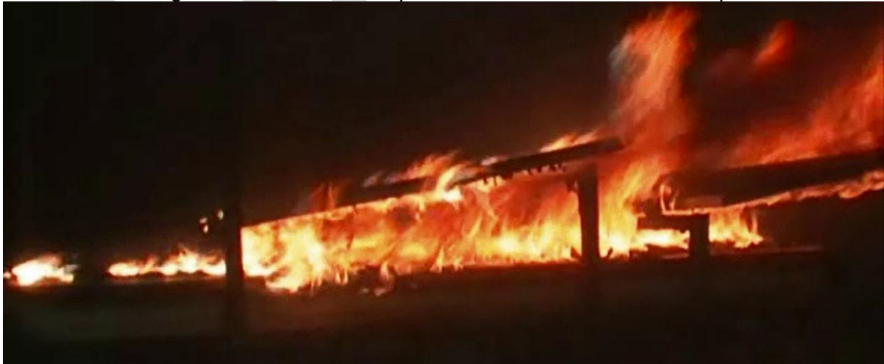
Figure 5 – Figure Illustrating Flame Spread of System 14 - Low Slope Roof / 2 PV Modules LSFR EPDM, 5" Gap, 10° Inclinations and First Module 24" Offset, Second Module Spaced 12" Experiment
