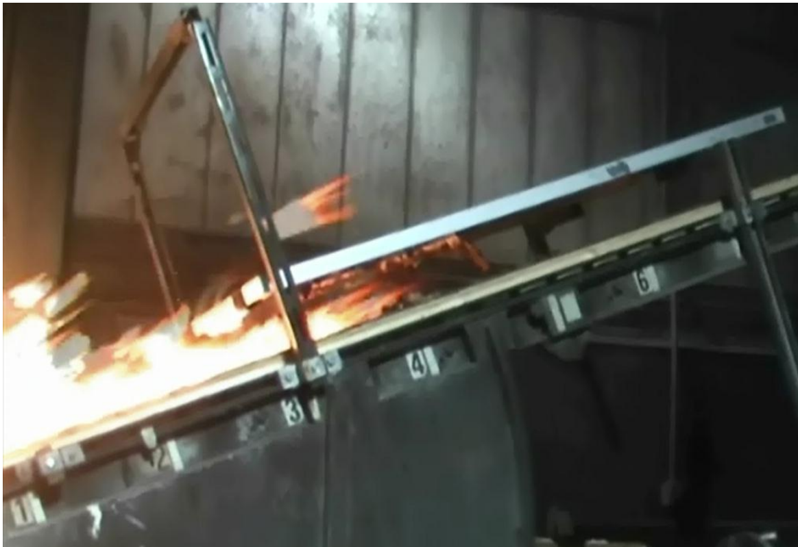
Figure 8 – Figure Illustrating Flame Spread of System 2 – Steep Slope Roof / PV Module Mfg. #1 Shingle, 5" Gap, 0° Inclination and 36" Offset Experiment
