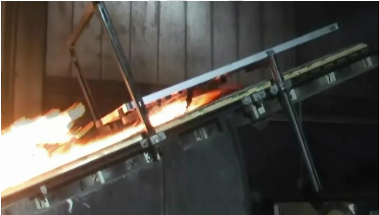
Figure 11– Figure Illustrating Flame Spread of System 8 – Steep Slope Roof / PV Module Mfg. #3 Shingle, 5" Gap, 0° Inclination and 36" Offset Experiment
