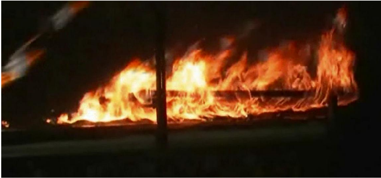
Figure 1 – Figure Illustrating Flame Spread of System 14 - Low Slope Roof / PV Module LSFREPDM, 5" Gap, 0° Inclination and 48" Offset Experiment
