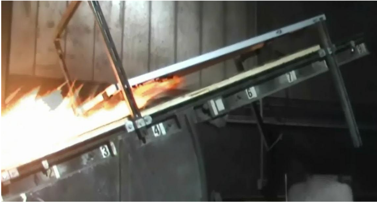
Figure 6 – Figure Illustrating Flame Spread of System 6 – Steep Slope Roof / PV Module Mfg. #1 Shingle, 5" Gap, 0° Inclination and 42" Offset Experiment
