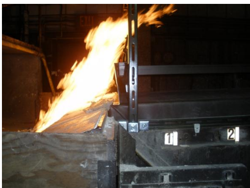
Figure 5 – Photograph of Flame with a the Opening Blocked by Flashing Installed on a Low Slope Roof Assembly
