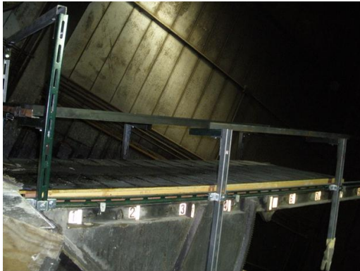
Figure 3 – Figure Illustrating Steep Slope Roof / PV Module Assembly 12” Gap Sample After Flame Spread Experiment
