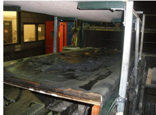
Figure 4 – Figure Illustrating Low Slope FR EPDM Roof / PV Surrogate Assembly 24” Gap After Flame Spread Experiment
