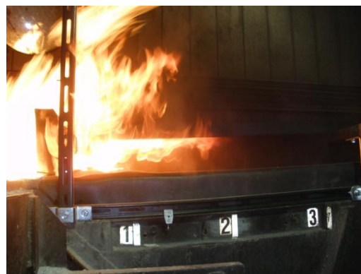
Figure 6 – Photograph of Flame with a ½ in. Flashing Opening Flashing Installed on Low Slope Roof Assembly
