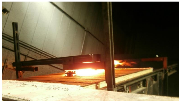
Figure 2 - Photograph of Brand Positioned Below the Module
