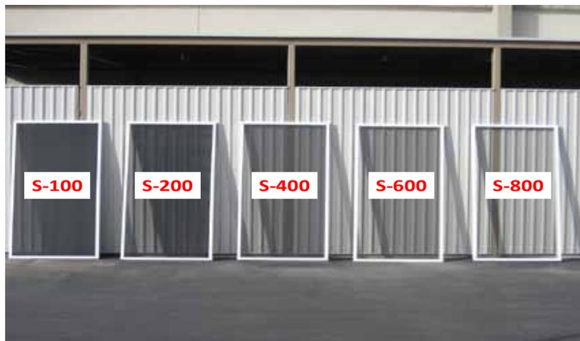
Figure A2. Mesh screens (100"x50") used in this investigation.
