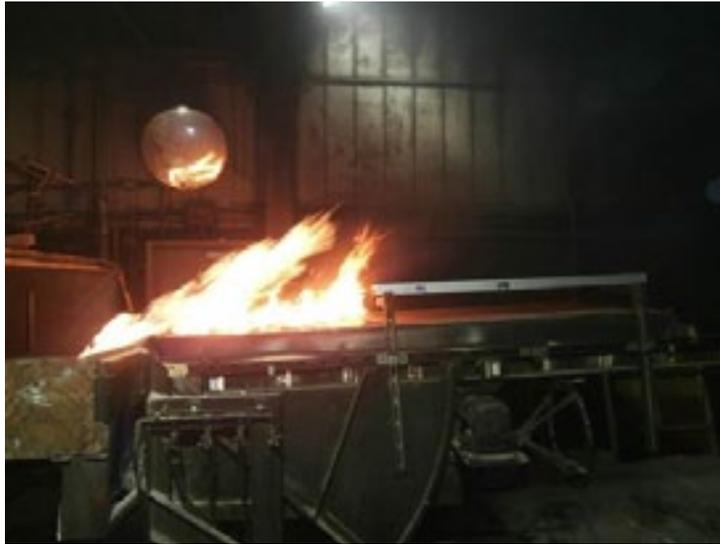
*Figure 5.* Example experiment illustrating first to ignite, second to ignite concept with 48-inch offset (low slope roof with low slope FR EPDM, noncombustible PV surrogate, five-inch gap)
