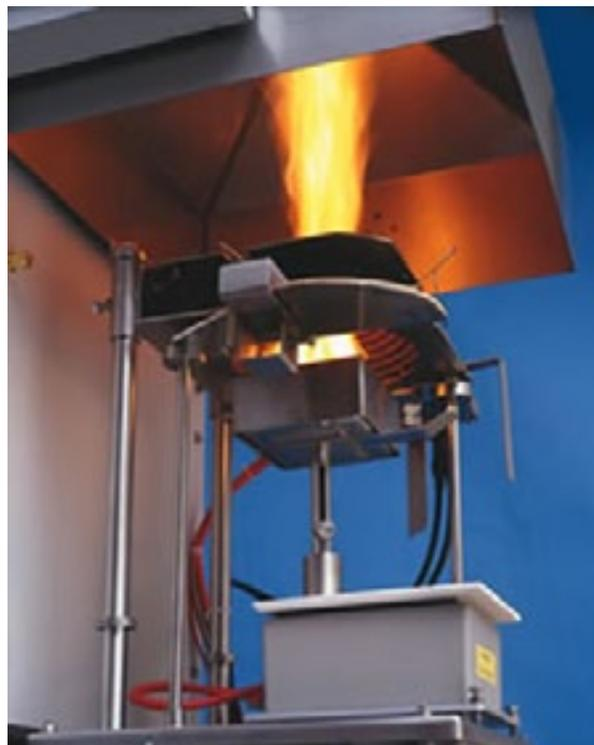
*Figure 4.* Cone calorimeter test apparatus (ASTM 1354).
