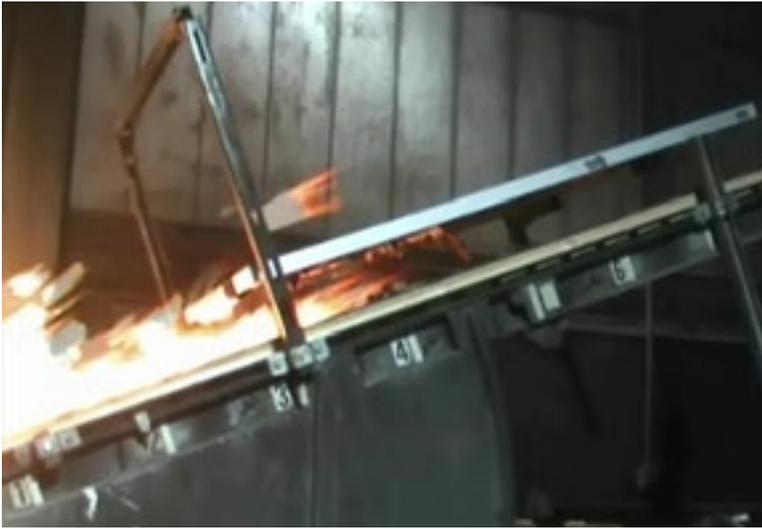
*Figure 6.* Spread of flame test with steep slope roof and PV module, 36-inch offset, five-inch gap, and 0° inclination.
