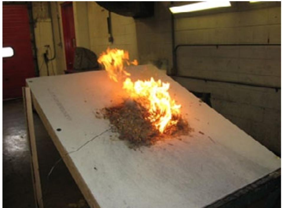
*Figure 3.* Experimental setup with leaf debris over noncombustible deck.
